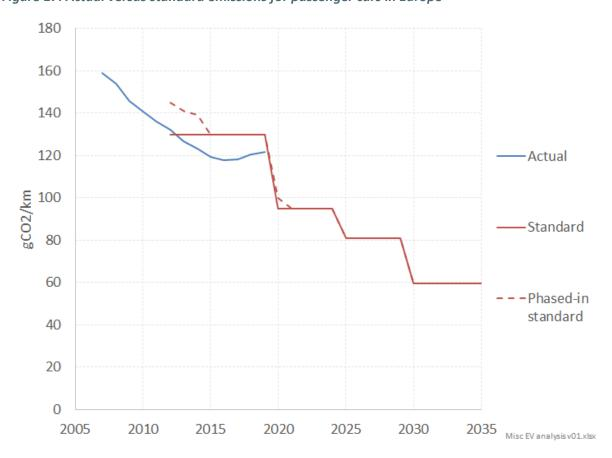
Figure 17: Actual versus standard emissions for passenger cars in Europe
